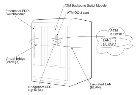
Figure 2-4 ATM Backbone SwitchModule LANE Components
